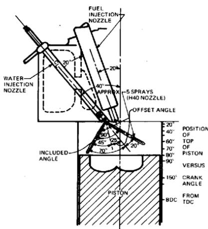
Fig. 2. Engine head and water injector location.
