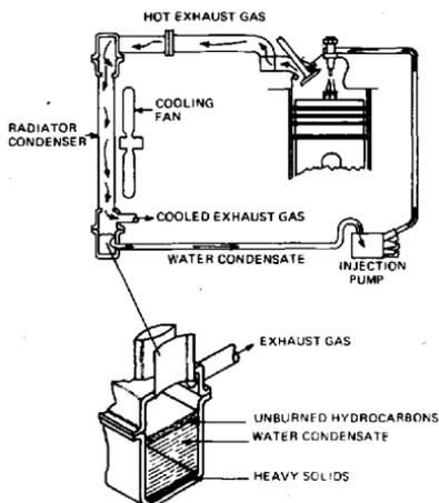
FIG. 1. Schematic illustration of water-injection condensate recycle concept.
