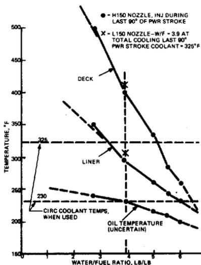
FIG. 7. Estimated equilibrium temperatures versus water/fuel ratio with head and liner coolant drained.
