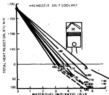
Fig. 3. Total Btu rejected versus water/fuel ratio—Numbers on curves are the end of water-injection timing, CA degrees from TDC power stroke.
